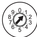
Figure 3.1: Address switch set to 1
