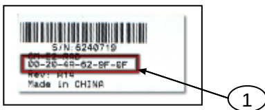
Figure 4: MAC Address Location
