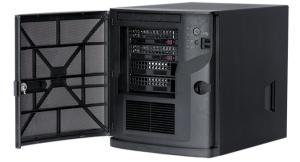
DIVAR IP all-in-one 4000 is an affordable and easy to use all-in-one recording, viewing, and management solution for network surveillance systems of up to 32 channels (with 8 channels pre-licensed). DIVAR IP all-in-one 4000 is a 2-bay mini tower unit that combines advanced Bosch Video Management System capabilities and state-of-the-art recording management into a single cost-effective, convenient to install and operate IP recording device for ITminded customers.
